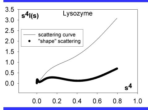
At larger s-values the scattering of a particle with  $\rho_s \neq 0$  oscillates around a straight line given by POROD's law:
