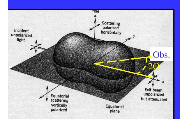
where  $2\theta$  is the angle between the incident and the scattered beam.
