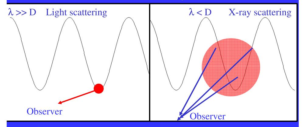
When  $\lambda >> D$  all N electrons in the particle are accelerated in phase the scattering amplitude is N times that of one electron.
