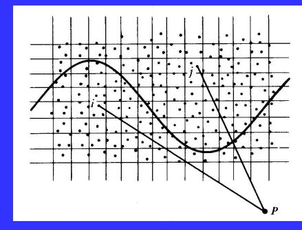
In a perfectly homogeneous body the contribution of each small scattering volume element to the scattering amplitude would always be cancelled out by that of another one which is out of phase. This is why perfect crystals do not scatter visible light.
