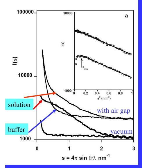
Background arises from the incoherent (Compton) scattering from the sample and from coherent and incoherent scattering due to air gaps, windows, solvent ....
