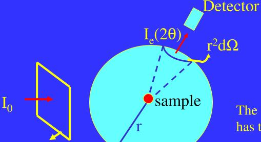
$$\frac{d\sigma}{d\Omega} = \frac{I_{e}(2\theta)}{I_{0}} \cdot r^{2} = |b|^{2}$$
